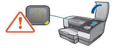
2 Open the printhead access latch by lifting the latch from the rear. Pull the latch forward and down to release the hook from the carriage lock.
